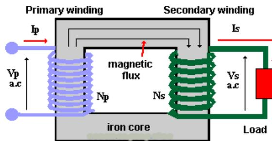
Figure 17: Working Principle of Transformer [16]
