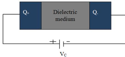
**Figure 12: Parallel Plate Capacitor**
