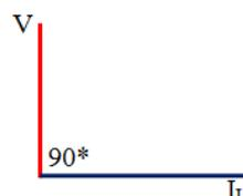
**Figure 3: V-I Curve for Pure Inductive Load**
