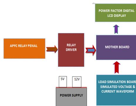
Figure 6: Block Diagram APFC
