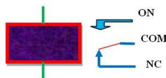
Figure 11: Circuit Symbol of Relay
